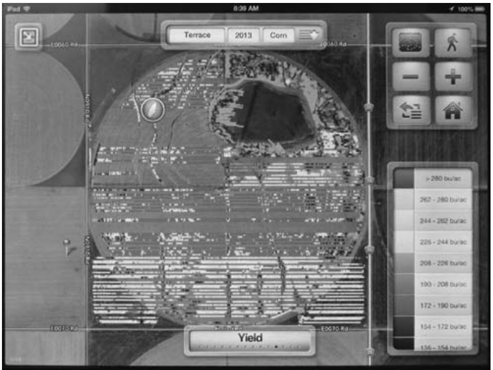
A screenshot of near real-time variable-rate irrigation (VRI) yield data on an iPad from the cab of a combine. The VRI system prevents the application of water on unproductive soils, such as the large spot in the photo above.
